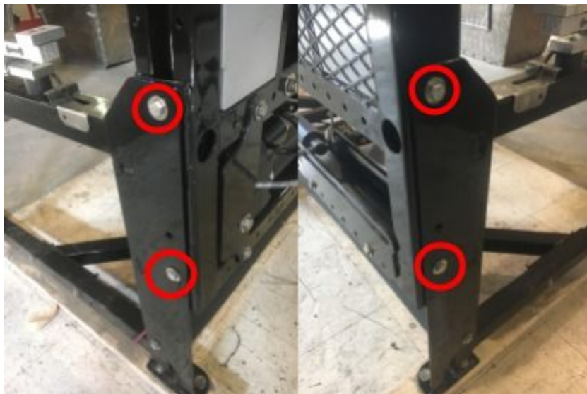
Figure 9) Loosen four bolts to raise/lower the front of SmartFeed
